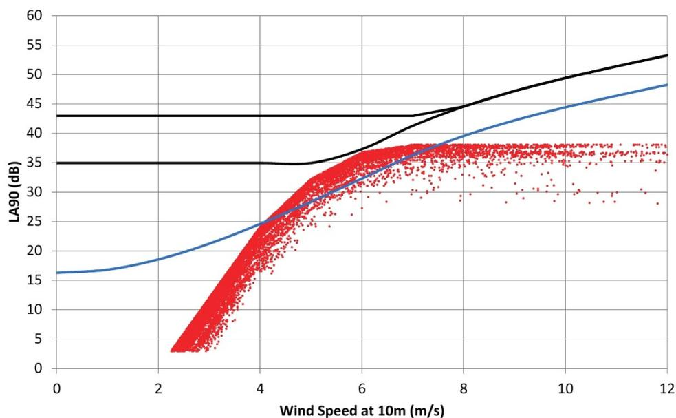
**Figure 8:** Predicted wind turbine noise based on the erroneous ETSU-R-97 assumption regarding wind shear. The red dots are wind turbine noise; blue line is night hours prevailing background noise curve and the two black lines are 35dB and 43 dB noise limits based on this background.
