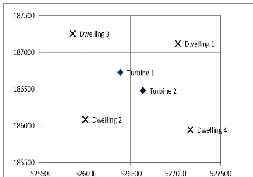
**Figure 6:** Hypothetical turbine and dwelling layout resulting in potential maximum turbine noise level assessed as 37.2 dB at dwellings 1 and 2, and 35.7 dB at dwellings 3 and 4.
