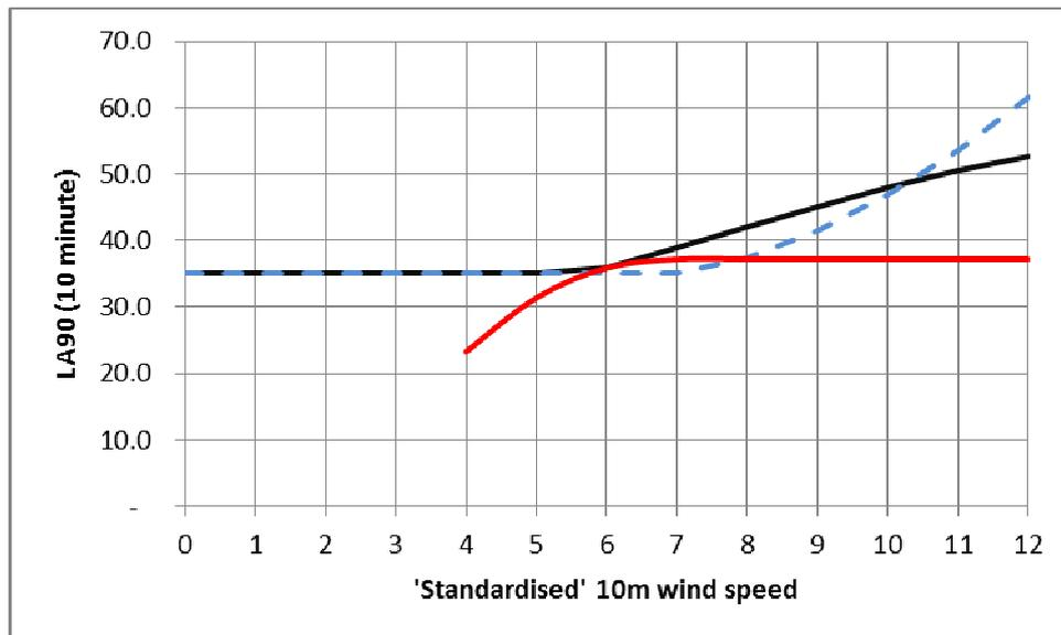
**Figure 5:** Red line gives turbine noise profile. The two amenity-hours noise condition profiles are obtained from the two different periods shown in Figure 4. The black line is amenity condition A, and the dashed blue line is amenity condition B.
