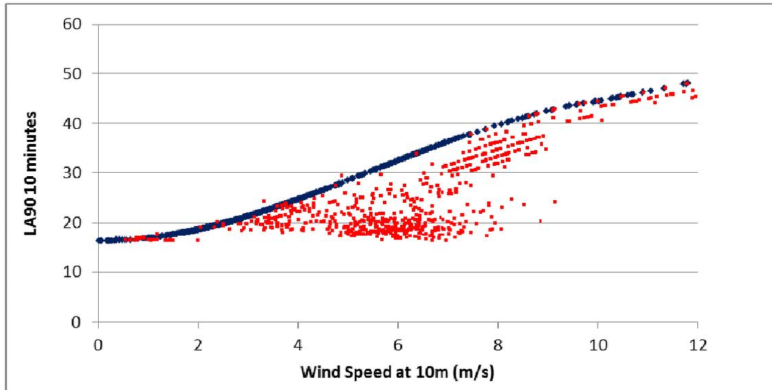
**Figure 2:** The blue points above show two weeks of an ETSU-R-97-type plot of average noise vs 10 metre wind speed. The red points are the same average noise data points vs the *Bulletin* method's transformed 10 metre wind speed (the so-called 'standardised' wind speed). The horizontal axis indicates the 10 metre wind speed for the blue points and a 'standardised' 10 metre wind speed for the red points.
