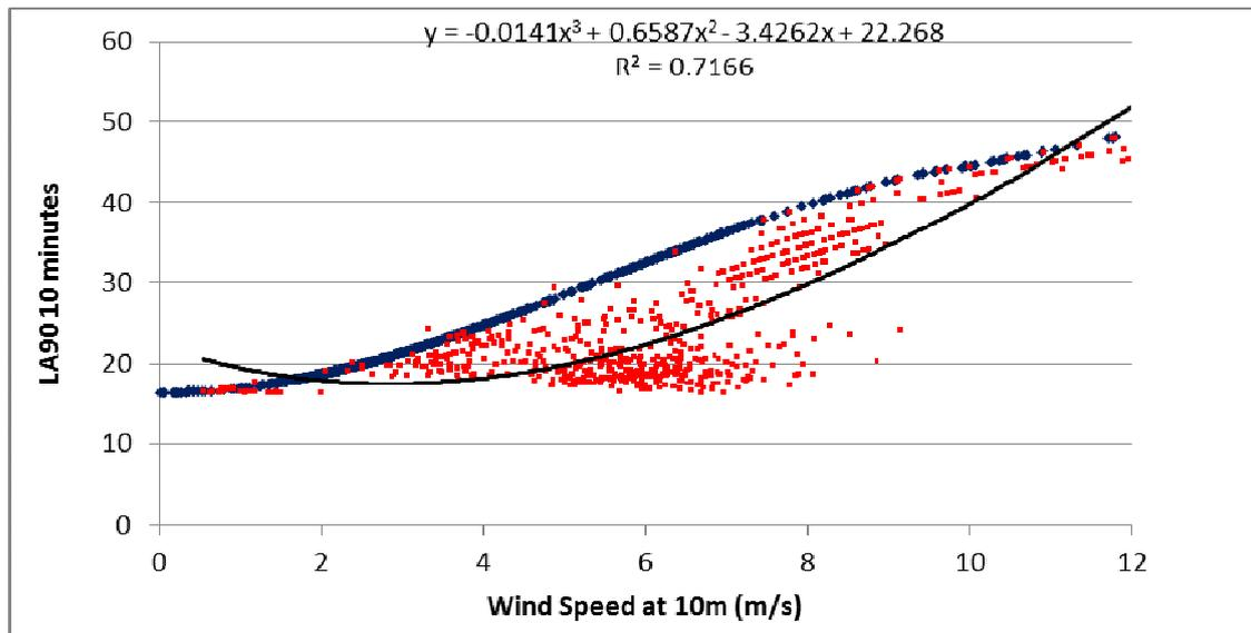
**Figure 3:** The data in Figure 2 with a best-fit third order polynomial (black line) fitted to the red Bulletin-methodology data.
