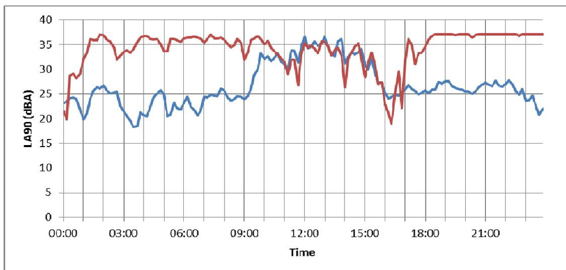
**Figure 7:** Average background noise (blue line) and turbine noise (red line) at Dwelling over all 24 hours of the 8<sup>th</sup> of February 2008). The periods of high wind shear during the evening and night result in an increased difference between the two noise levels, resulting in an increased probability of complaints.
