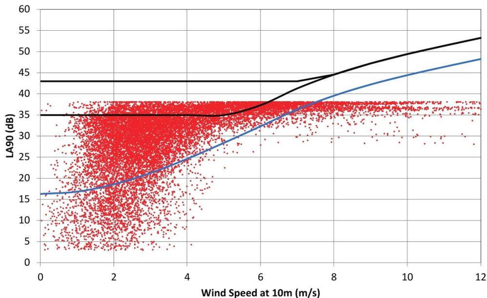
**Figure 9:** Predicted wind turbine noise based on actual wind shear. The red dots are wind turbine noise; blue line is night hours prevailing background noise curve and the two black lines are 35dB and 43 dB noise limits based on this background.
