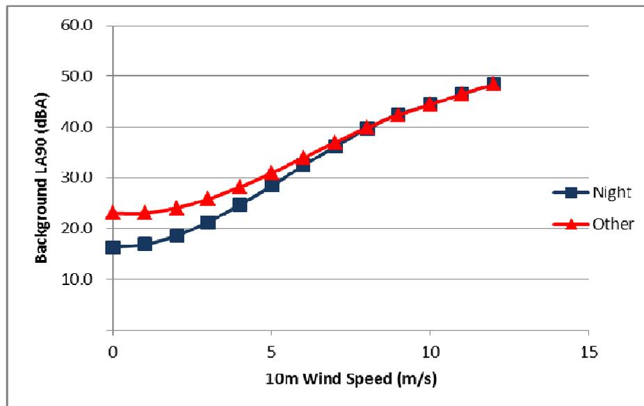
**Figure 1:** The two selected profiles chosen to represent average background noise vs 10 metre wind speeds for Night times (11 pm to 7 am) and all other times.
